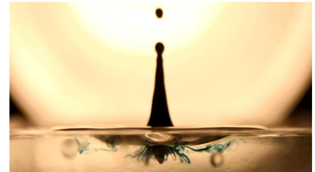
Drop impact flow components: splash with ejected drop, cavity and crown remnants, ligaments (loops), capillary waves
