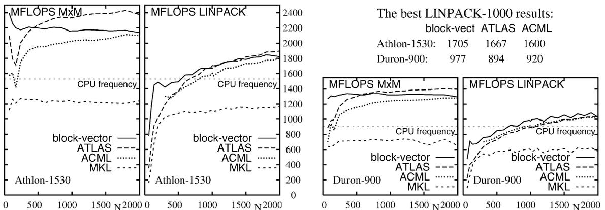
Fig. 6. Performance of different algorithms for matrix multiplication (left plots) and solving linear systems (right plots) on Athlon-1530 and Duron-900 processors.
