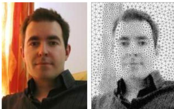
*The left [picture](#) was used to determine the size of the triangles in the [mesh](#) shown on the right. The triangulation was done with [Gmsh](#) using this [script](#).*
